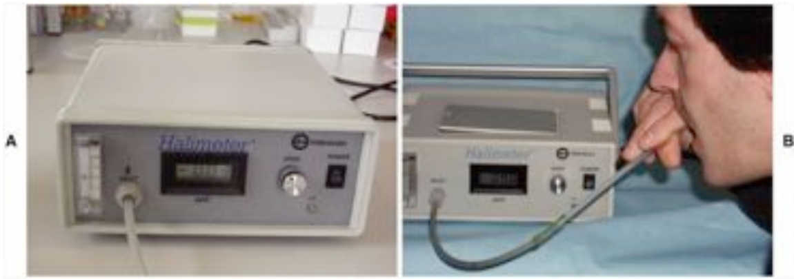
A , Portable sulfide monitor. B , Patient holds the aspirating tube in his mouth. Digital reading reveals the total amount of volatile sulfide compounds (VSCs) in parts per billion (ppb).
