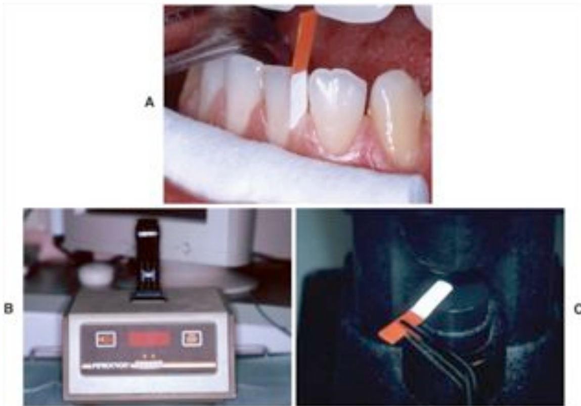
Sampling method for gingival crevicular fluid (GCF) analysis (Periotron). A , Saliva is removed from the tooth surface with cotton wool before placement of a periopaper strip into the pocket to collect GCF. B , The moist paper strip is removed and placed between the jaws of the Periotron for assessment of fluid content. C , Periotron device.
