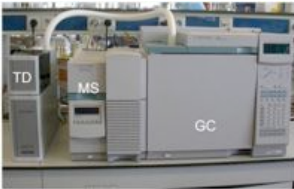
Gas chromatography machinery, including thermodesorber ( TD , to release molecules trapped in special collectors), gas chromatograph ( GC , for separation of molecules), and mass spectrometer ( MS , for identification of molecules).
