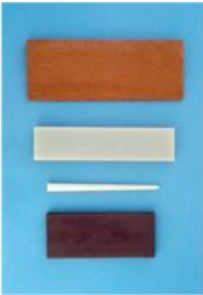
Sharpening stones. Top to bottom , A flat India stone, a flat Arkansas stone, a cone-shaped Arkansas stone, and a ceramic stone.
